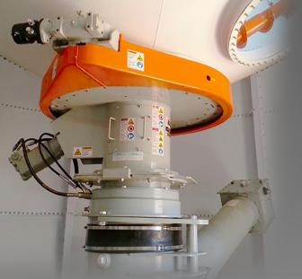
Laidig's **Cone-Bottom** reclaim systems are designed specifically for reclamation of materials with poor-flow characteristics or other properties which make the material difficult to handle.
